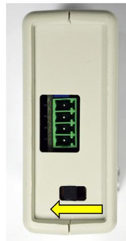
RS232/485 switch is located on the side of chassis box. The black slide switch needs to be positioned to the left as shown (or positioned to the top of the device if not on its side).
